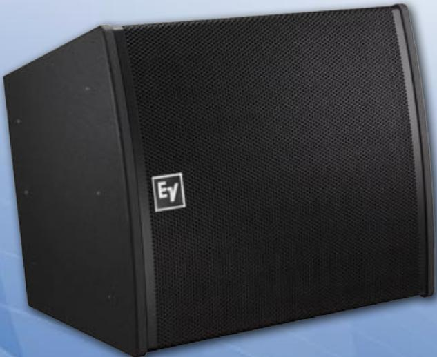
Each full-range EVA module has a sophisticated internal crossover network and a nominal impedance of 16 ohms, allowing (for example) an entire four module (eight element) array to be driven by a single amplifier channel as a 4 ohm load.
